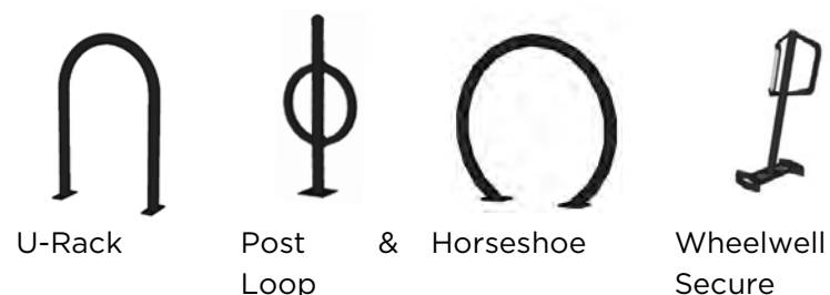
Figure 3-2: Types of bicycle racks
