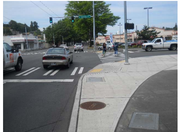
Figure 28. Narrowed curb radius
