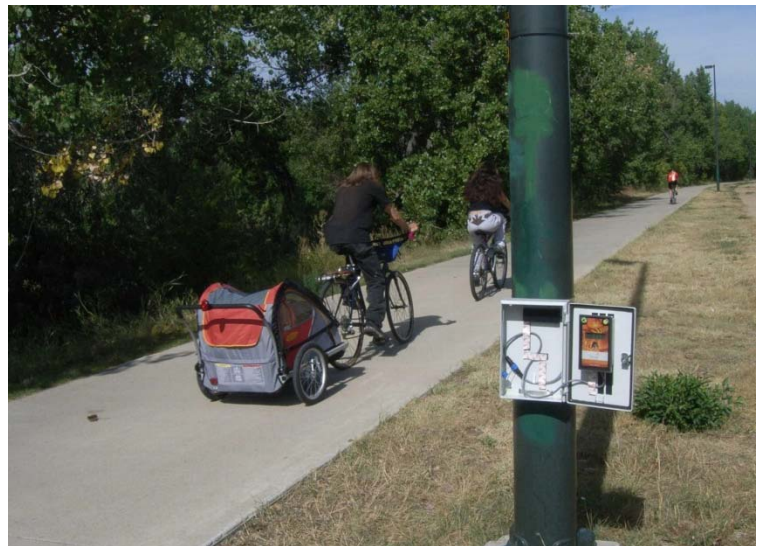
Figure 21. Infrared counter on multi-use trail in Denver, CO. Credit: Colorado Department of Transportation.
