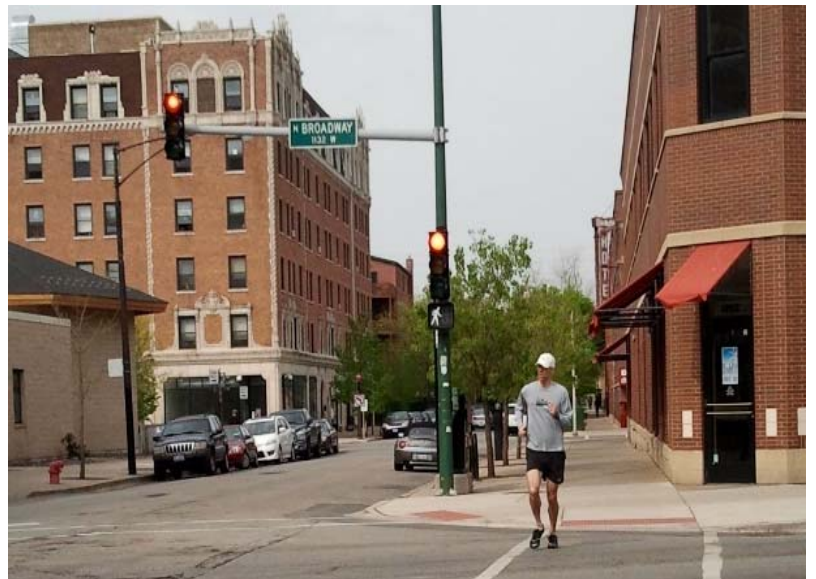
Figure 43. Leading Pedestrian Interval. Note that the pedestrian has been given the “Walk” signal prior to giving the motor vehicles the green indication.
